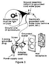
Grounded, cold water pipe must have Grounded, cold water pipe must have metal continuity to electrical ground and not be interrupted by plastic, rubber, or other electrical insulating connectors such as noses, fittings, washers or gaskets (including water meter of pump). Any electrical insulating connector should be jumped as shown with a length of No. 4, copper wire securely clamped to bare metal at both ends.
